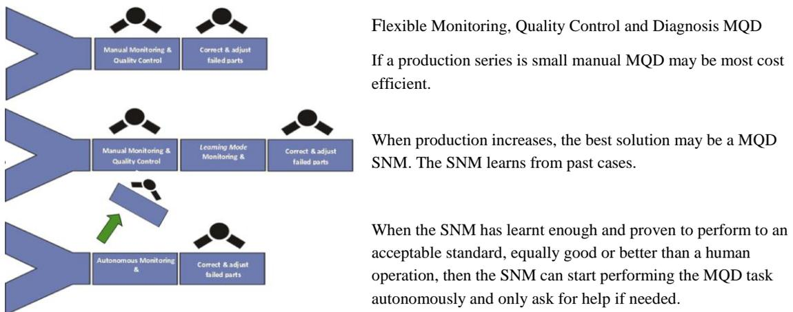
**Figure 12: Example for Flexible Monitoring, Quality Control and Diagnosis**
