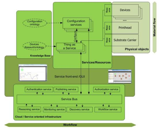
Figure 6: CREATE high-level architecture
