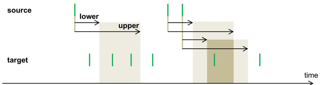
Figure 4. A set of event occurrences satisfying a DelayConstraint. Note the stray target occurrences outside the bounds set by the constraint.
