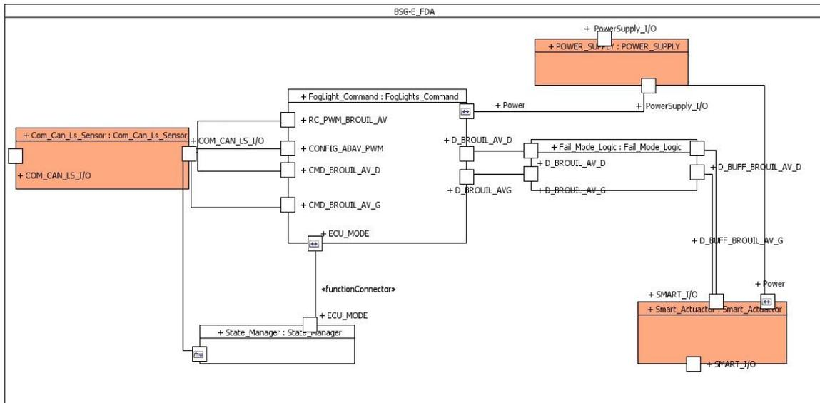
Figure 28. Functional Design Architecture of the BSG-E System.
