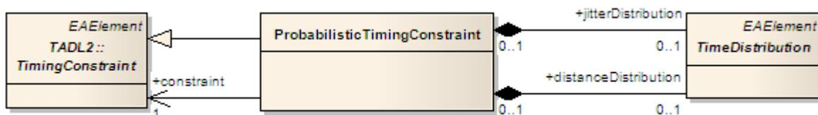
Figure 41: Constraints for probabilistic timing modifies timing constraints and add a distribution.
