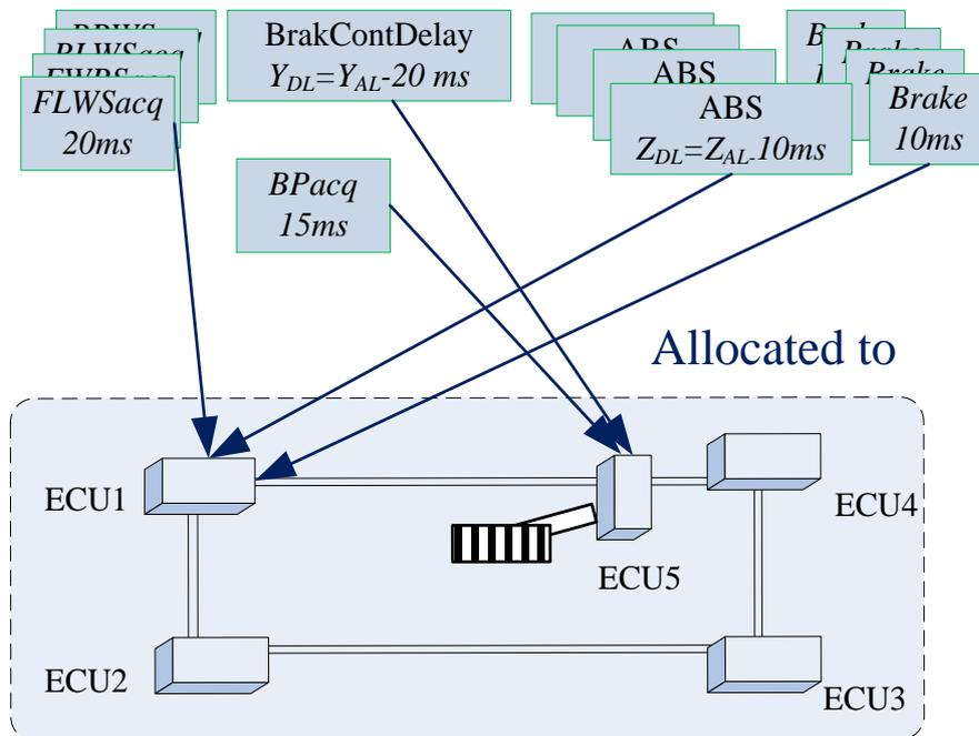
Figure 26. Hardware Architecture and Allocation of BBW Functions.
