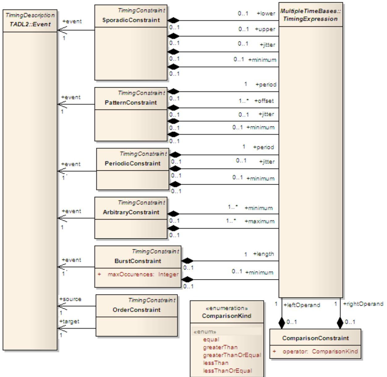
Figure 36: The second of two sets with TADL2 constraints with attributes of type TimingExpression and references to events. Also shown is the ComparisonConstraint with attributes of type TimingExpression.
