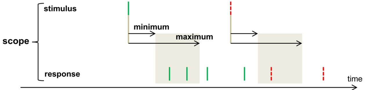
Figure 17. A set of event occurrences satisfying a ReactionConstraint. Causally connected event occurrences are shown by the same line style. Two sets are shown, one by a solid line and one by a dashed line.
