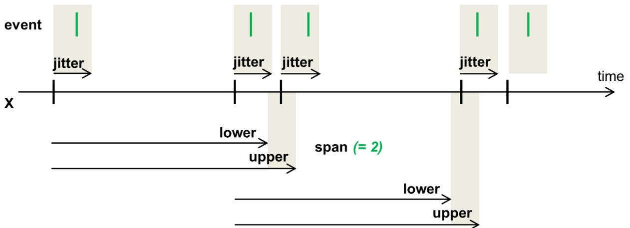
Figure 7. A set of event occurrences satisfying a RepetitionConstraint with a span of 2.
