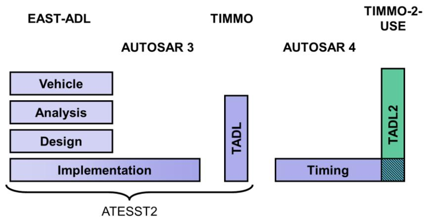
Figure 3. This figure shows how TADL and TADL2 spans the abstraction levels of EAST-ADL where AUTOSAR is available in the implementation level. AUTOSAR 4 includes a timing extension.
