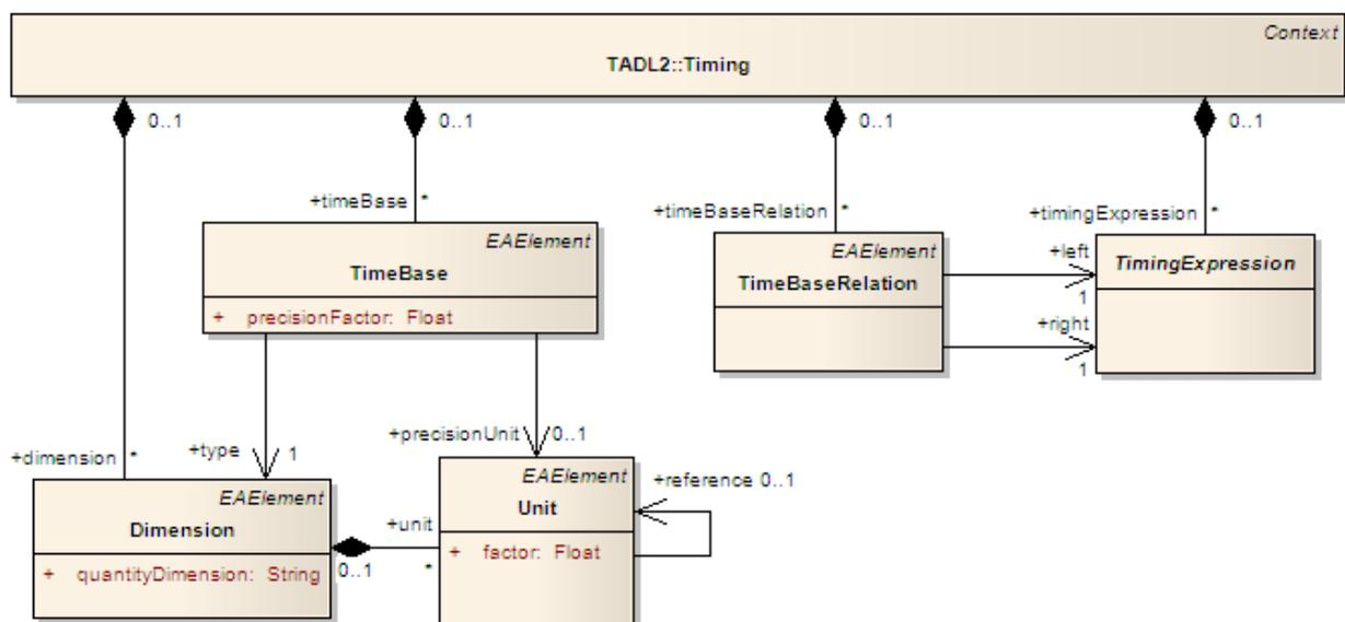
Figure 39: TimeBase with Dimension and Unit.
