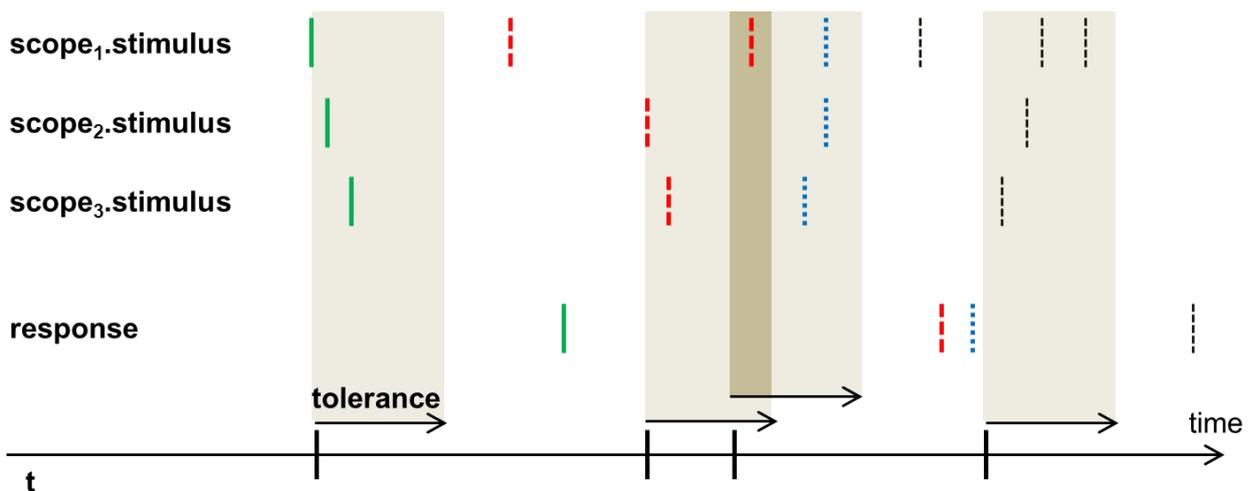
Figure 20. A set of event occurrences satisfying an InputSynchronizationConstraint. Stimuli event occurrences that are causally connected to a specific response event occurrence are shown by the same line style as the response event occurrence. Four sets are shown with different line styles.
