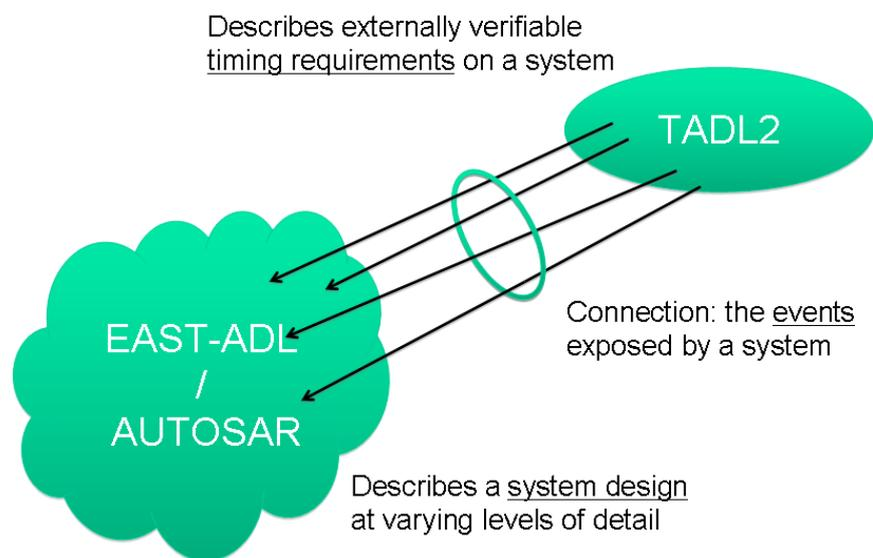
Figure 1. Events connect TADL2 to the system design modeled with EAST-ADL and AUTOSAR.
