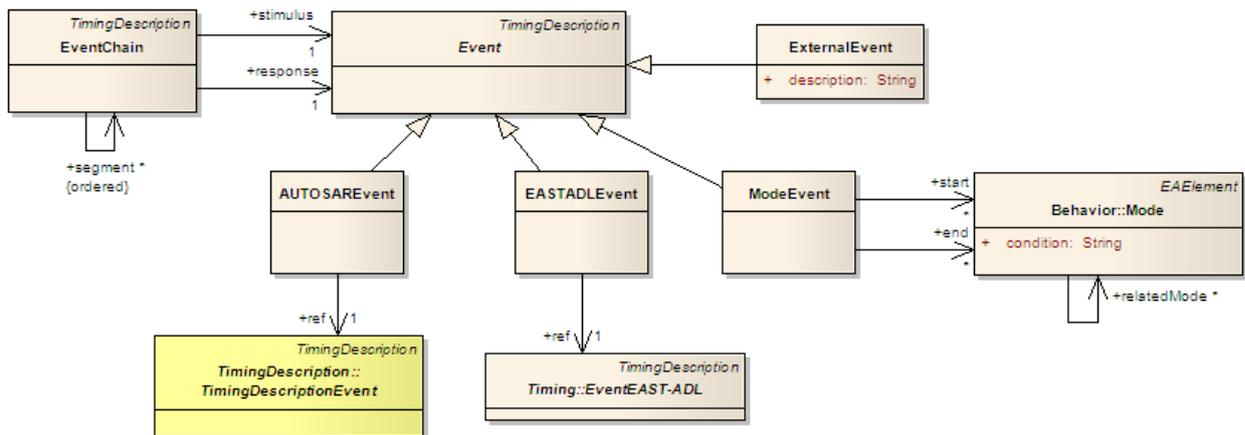
Figure 34: The Events are defined within AUTOSAR and EAST-ADL. These events refer to the structural models of AUTOSAR and EAST-ADL respectively.
