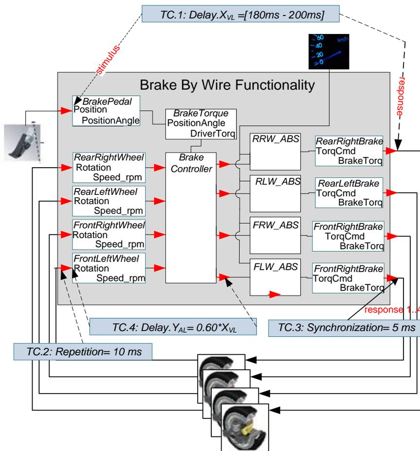
Figure 25. Brake-By-Wire Functional View.
