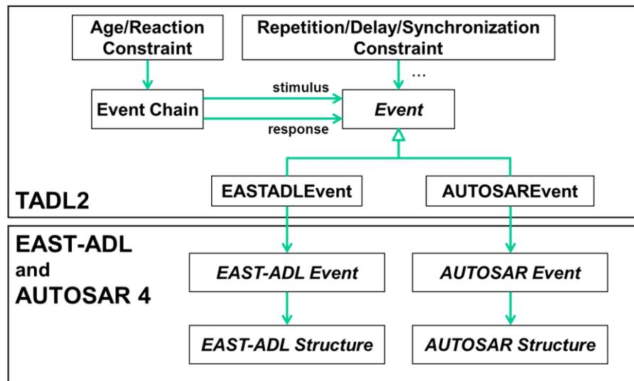
Figure 2. Different events are defined to refer to structural elements of EAST-ADL and AUTOSAR.
