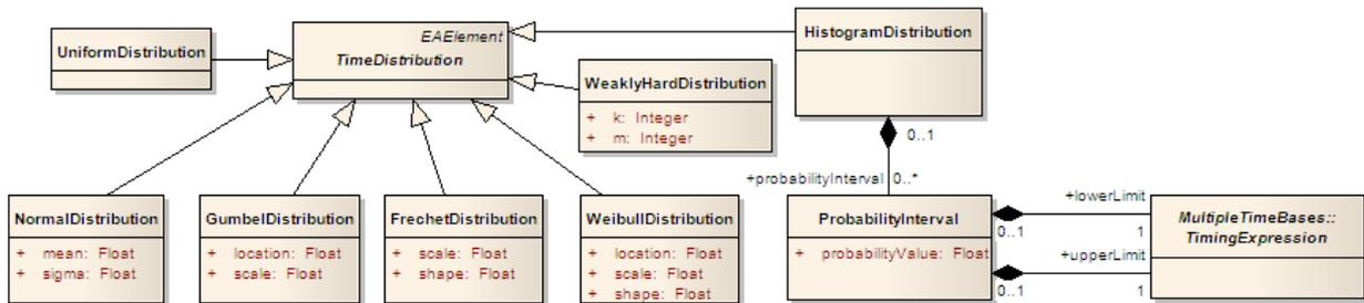
Figure 40: Distributions for probabilistic timing.
