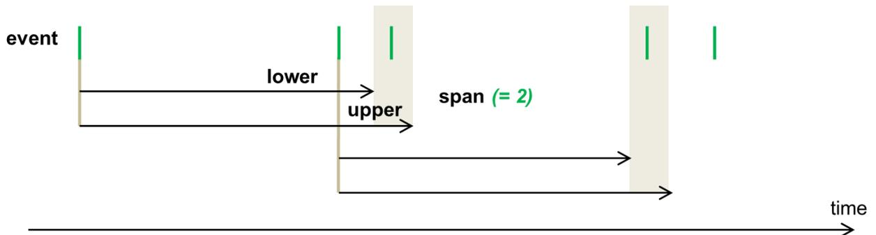
Figure 6. A set of event occurrences satisfying a RepeatConstraint with a span of 2.
