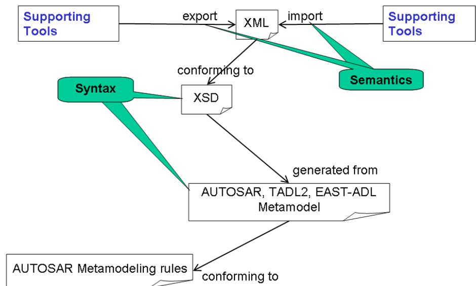
Figure 30. Tools operating on TADL2 use XML as exchange format.
