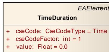
Figure 31: EAST-ADL metamodel for Units in timing constraints.
