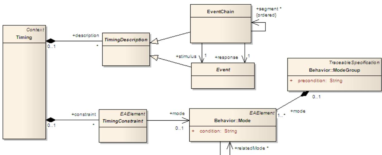
Figure 33: Basic TADL2 elements organized in Timing, with TimingConstraints referring to EAST-ADL Mode.
