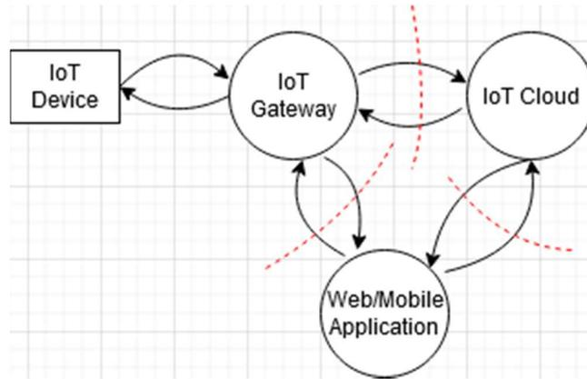
**FIGURE 2: AN EXAMPLE DFD DESCRIBING AN IOT ARCHITECTURE (SIMPLIFIED) - DFDs CAN BE USED TO SYSTEMATICALLY IDENTIFY THREATS/RISKS IN SOFTWARE AND SYSTEM ARCHITECTURES, RESPECTIVELY.**
