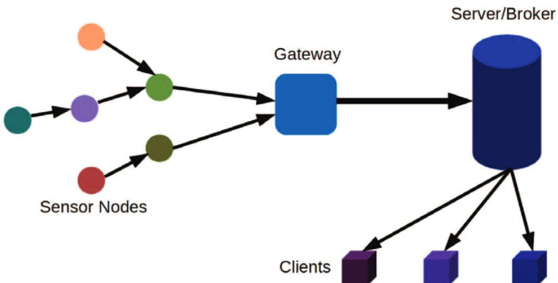
Figure 1. Wireless Sensor Networks
