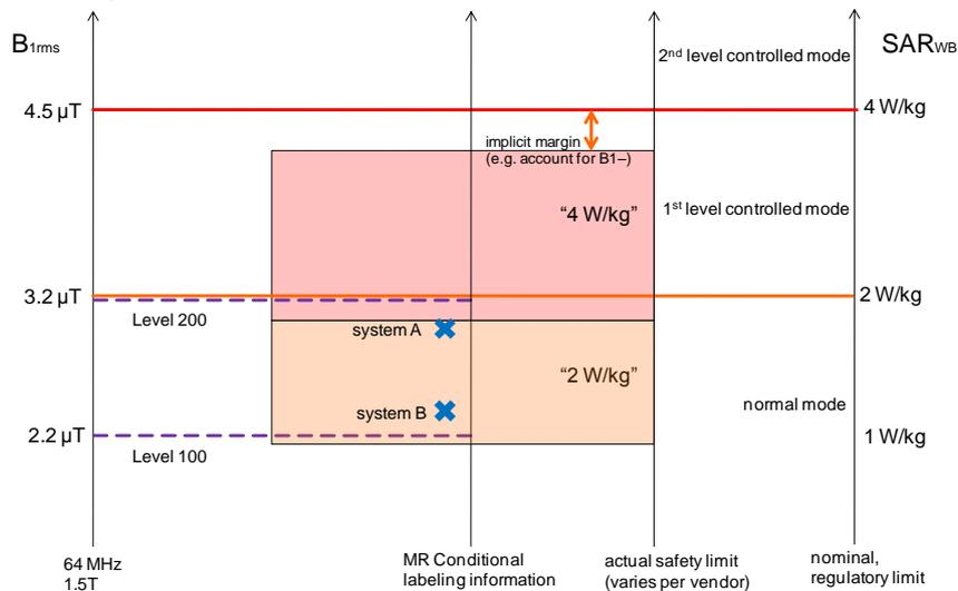
Figure 4. Schematic representation of (1.5T)  $B_{1rms}$  values and corresponding WB SAR values for typical body coil designs. Reported 2W/kg may result in significantly different actual deposited powers for different systems. Further margins may be applied by MR manufacturers to account for e.g.  $B_1^-$  contributions. Body Coil designs affect the conversion between  $B_{1rms}$  and WB SAR.
