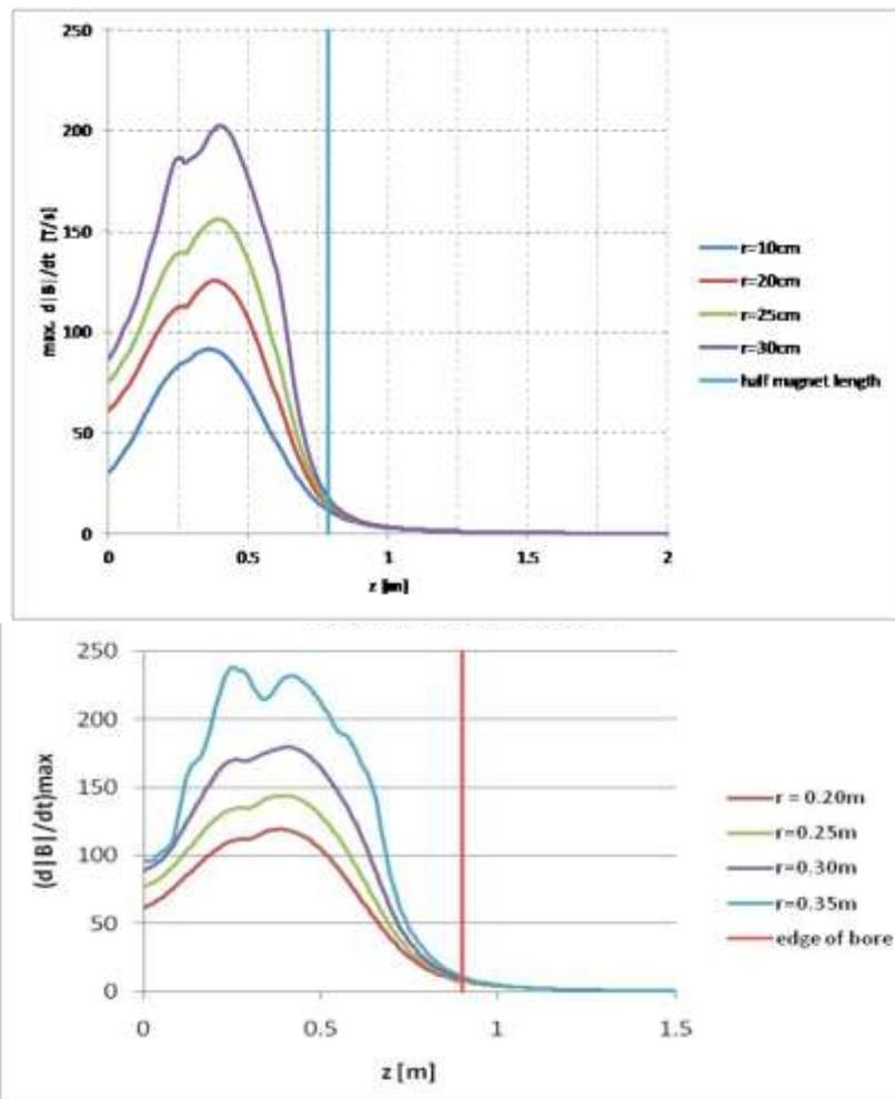
Figure 1. Graphs showing the maximum  $d|B|/dt$  at different radii around the central line of the bore of the MR system, for 60 cm, 40 mT/m, 200 T/m/s (top), and for 70 cm, 33 mT/m, 200 T/m/s (bottom).
