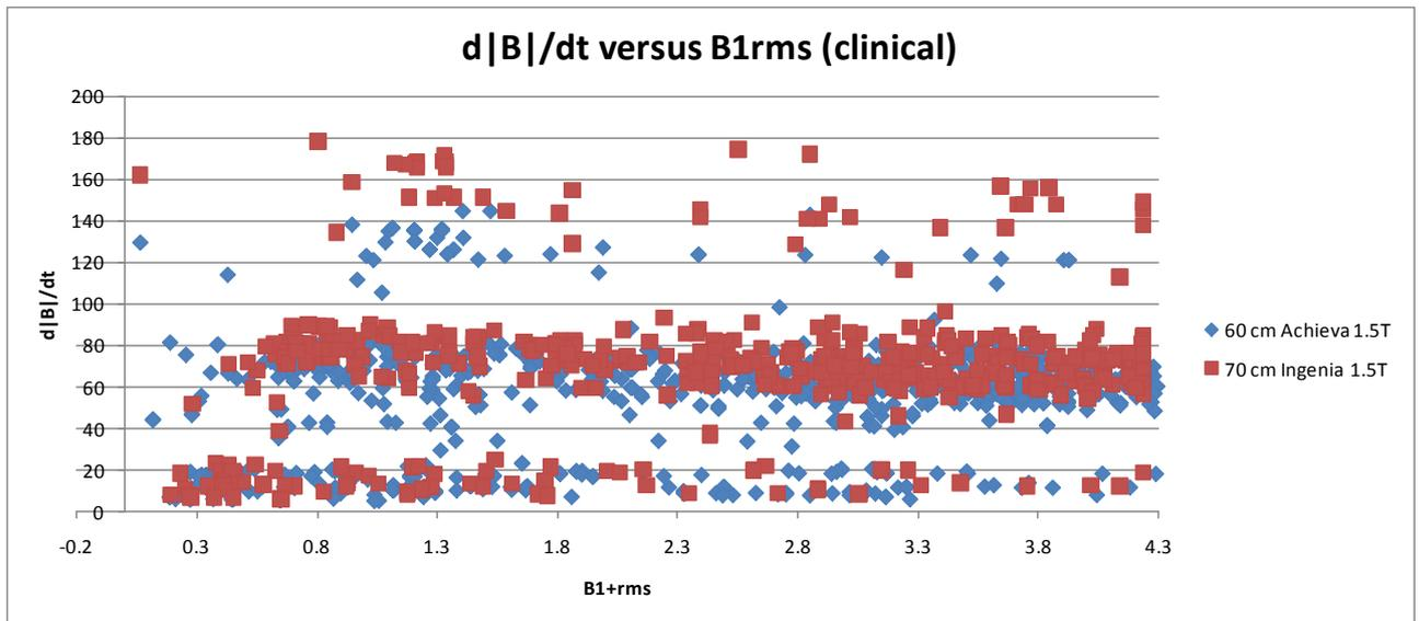
Figure 5. Scatter plot of calculated  $d|B|/dt$  values versus  $B_1^+_{RMS}$  for factory clinical sequences delivered with 60 cm and 70 cm MR systems. The orange dotted line indicates the allowed range of sequence parameters. A significant number of protocols (esp. TSE and bFFE), running in 1<sup>st</sup> level controlled mode, are (obviously) excluded by FPO, and need re-evaluation.
