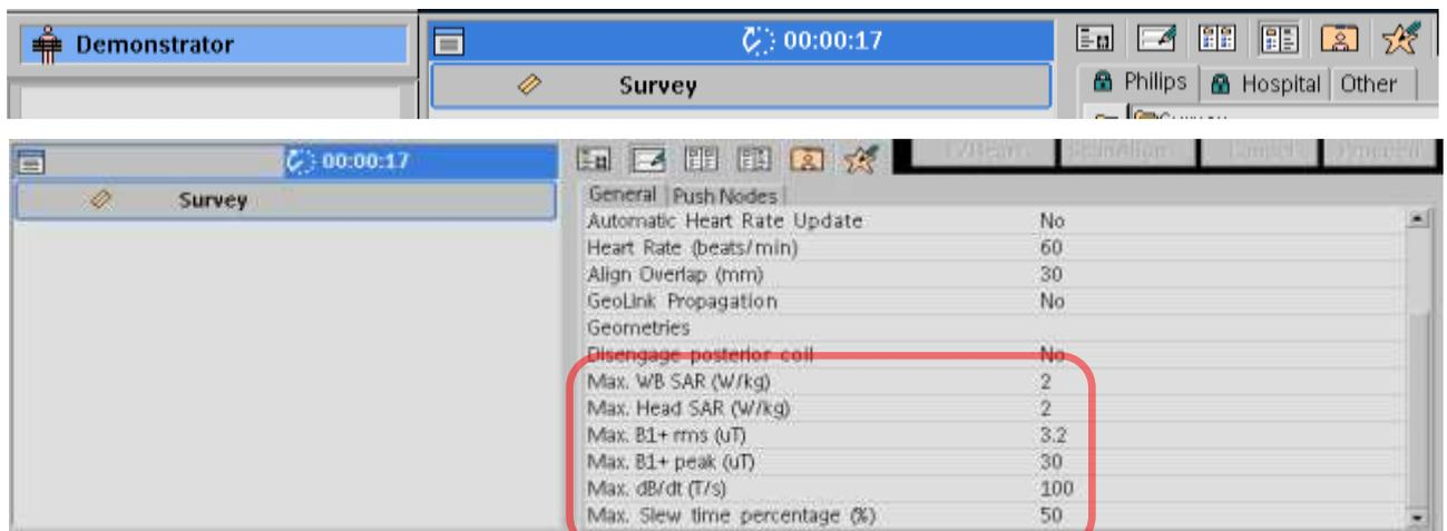
Figure 7. ExamCards User Interface screenshot of the Philips MR system, to illustrate the controls for the parameters defined in FPO. The user can define lower limit values for research and evaluation purposes.
