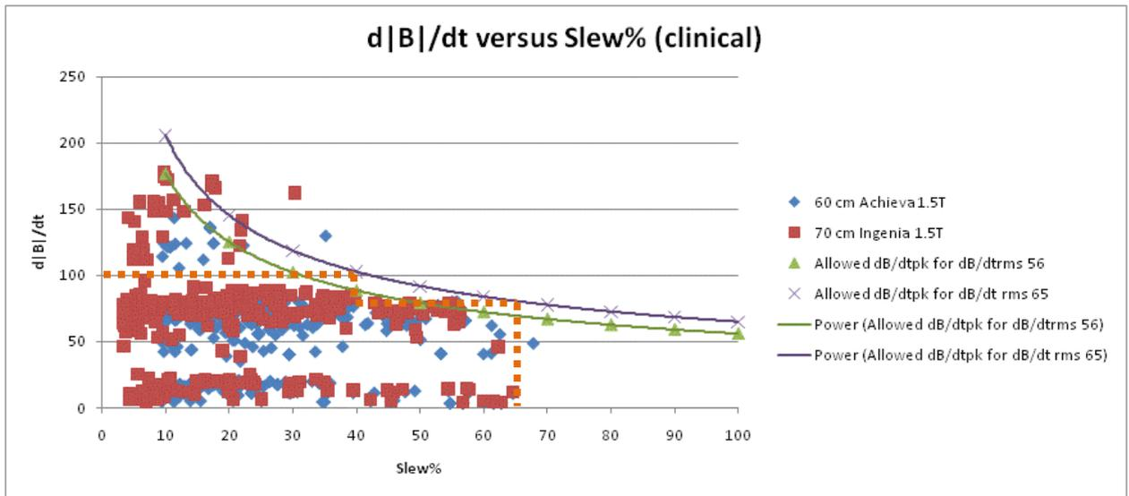
Figure 3. Scatter plot of calculated  $d|B|/dt$  values versus sequence slew-time percentages for factory clinical sequences delivered with 60 cm and 70 cm MR systems. Trend lines show the allowed  $d|B|/dt$ (peak) for two proposed limit values for  $d|B|/dt$ (rms), viz. 56 and 65 T/s. The orange dashed line indicates the proposed limits for clinical sequences in FPO.
