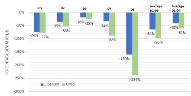
*Figure 9. Abatement percentage of OPC technology equipment compared with gravimetric equipment*
