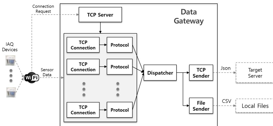
Figure 21. Data Gateway Architecture
