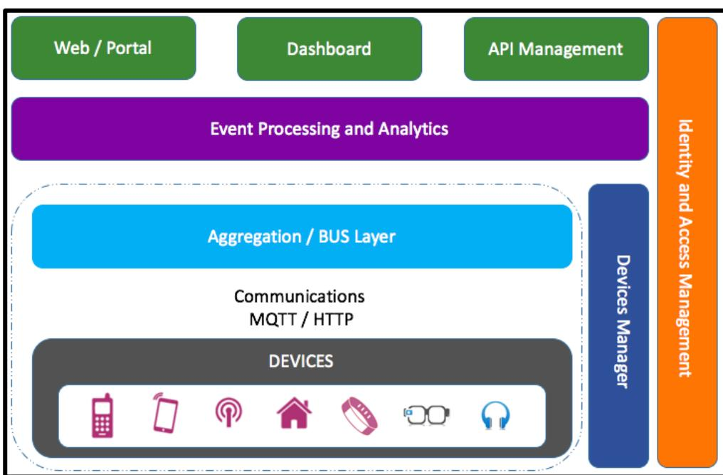
*Figure 27. Logical Layers of Establish Project from implementation point of view*
