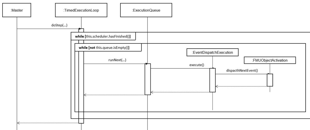
Figure 10 - Request a doStep on an FMU
