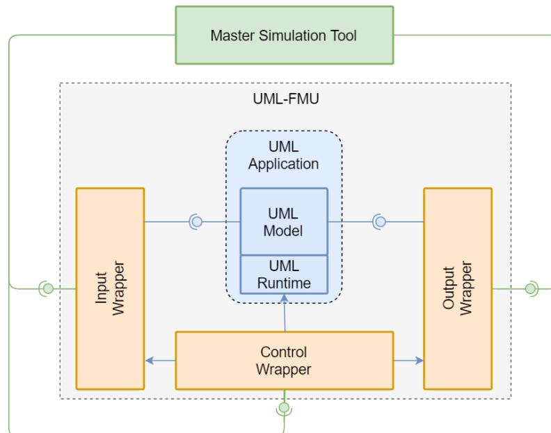
Figure 12 - Proposal to wrap a UML application model in a FMU
