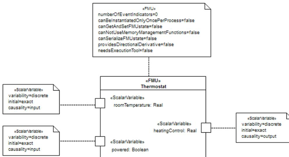
Figure 4 - Thermostat FMU defined with UML and the FMI profile
