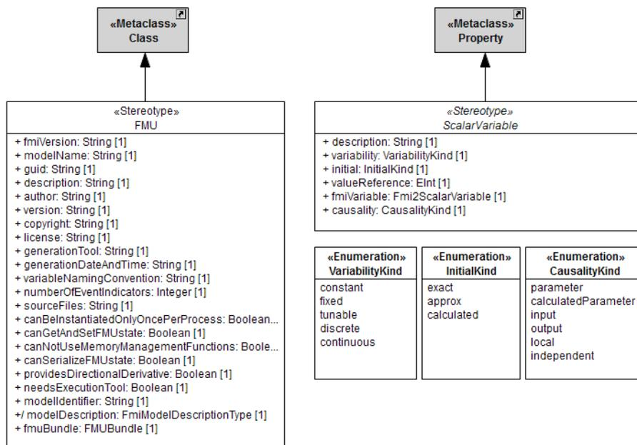
Figure 3 - Excerpt of a UML profile for FMI
