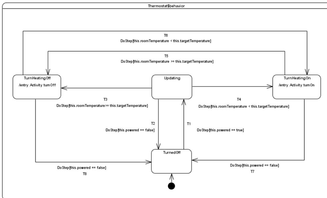
Figure 13 - Every transition is triggered by `DoStep`
