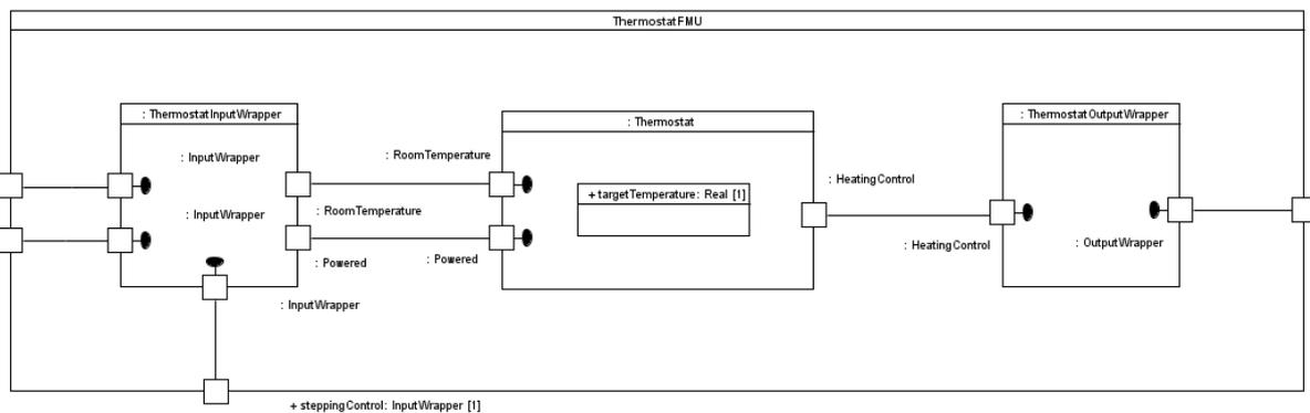
Figure 25 - Ports Typed by Interfaces - Wrapped Model
