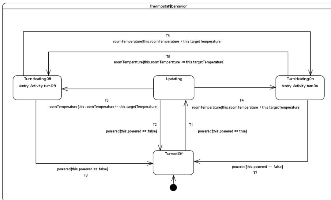
Figure 2 - Behavior specification of Thermostat FMU
