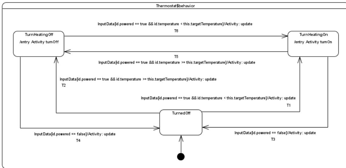
Figure 14 – Every transition is triggered by InputData
