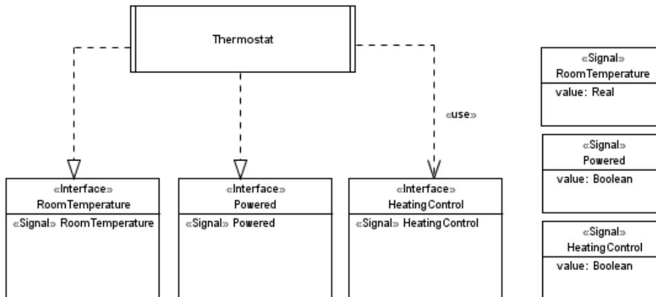
Figure 16 - Provided and Required Signals
