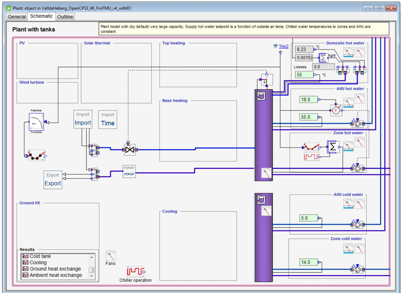
Figure 11. The model's plant, together with Import and Export components used by the FMU for communication
