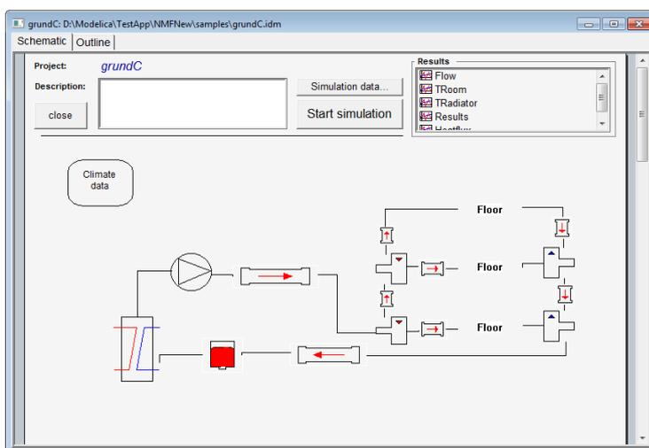
Figure 3.1. GrundA extended to three floors with 5 zones per floor.
