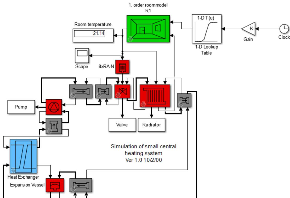
Figure 1. The GrundA Simulink model
