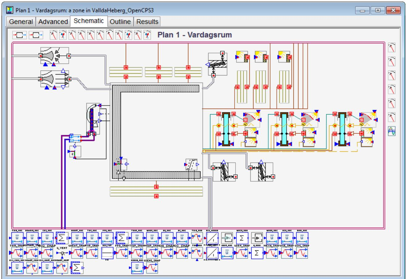
Figure 10. The model of one of the rooms in IDA ICE
