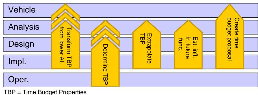
Figure 14 - The degree of presence of Find and Analyze timing properties tasks at different abstraction levels
