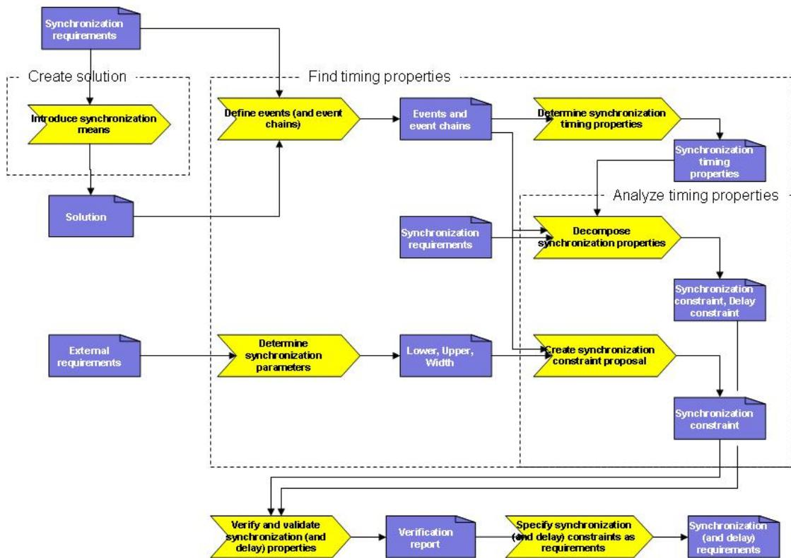
Figure 16 - Generic methodology for formulating and decomposing synchronization constraints
