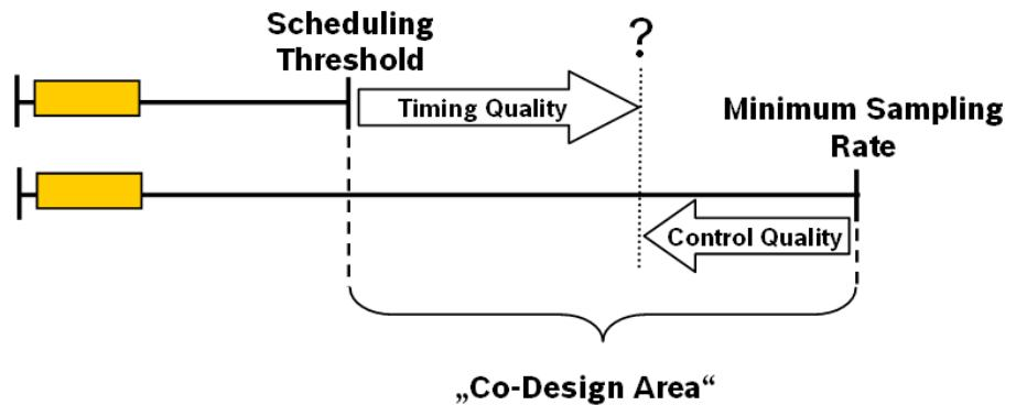
Figure 21 - Co-design area between control engineering and real-time engineering
