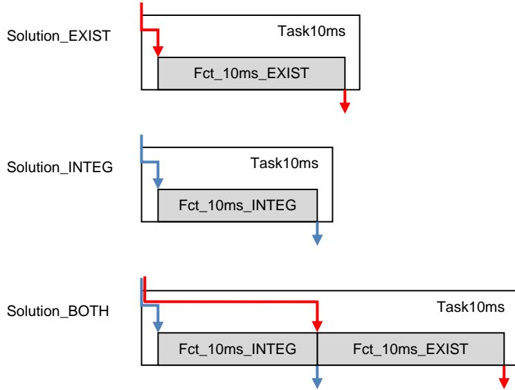
Figure 10 - Timing behavior before and after integration
