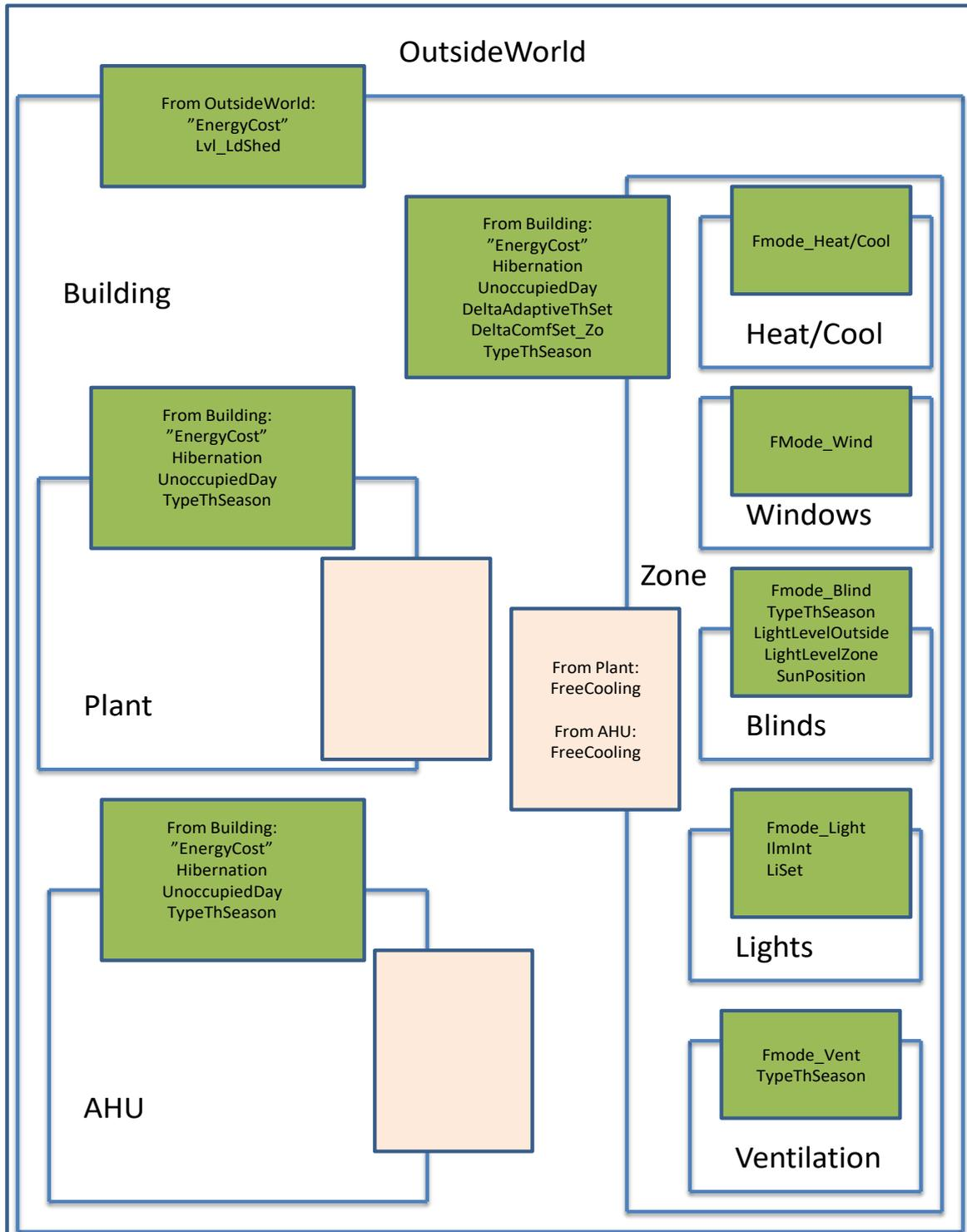
Figure 2 - Standard controller roles and signals.
