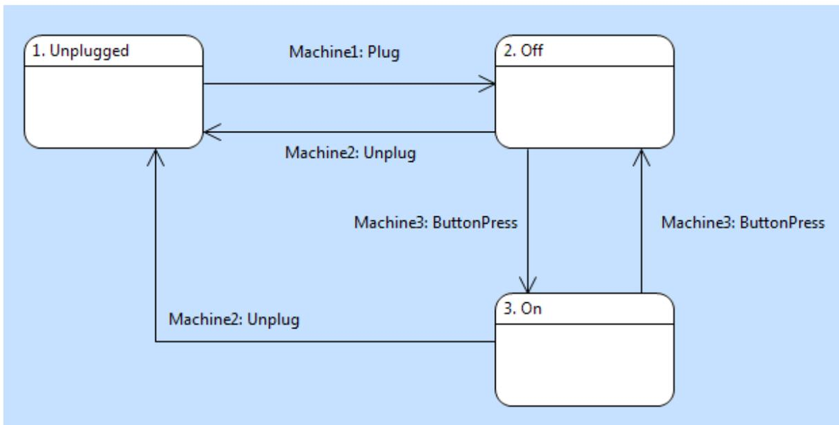
Figure 16 - An xtUML State Machine
