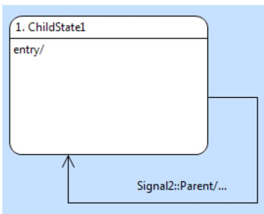
Figure 25 - State Machine of the Child Class
