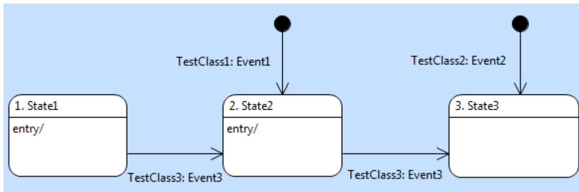
Figure 17 - State Machine with Creation Transitions
