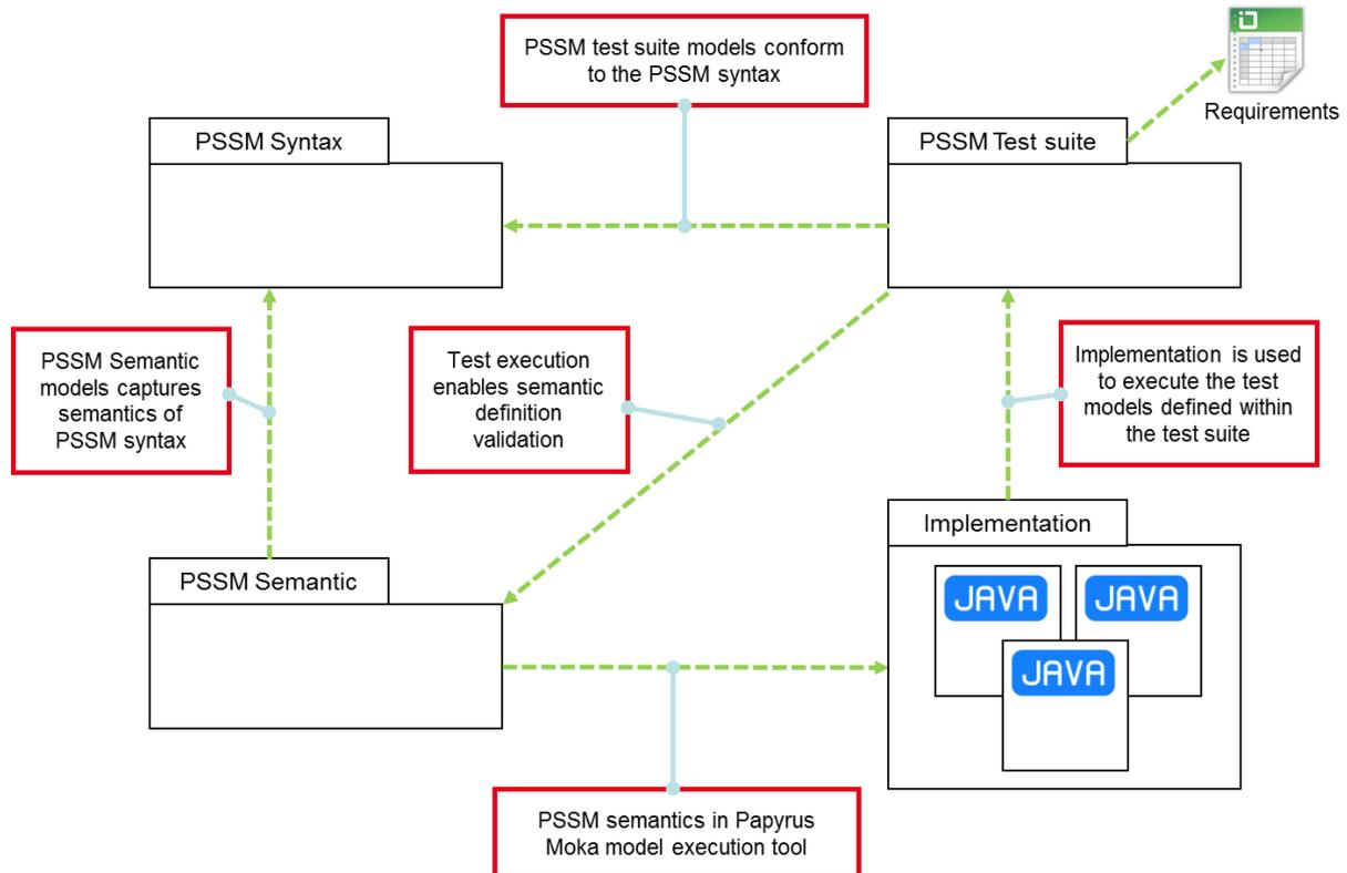
Figure 2 - PSSM specification architecture
