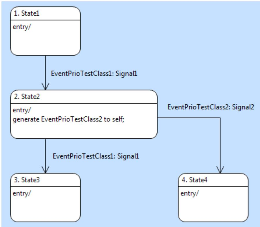
Figure 20 - State Machine with Self Event
