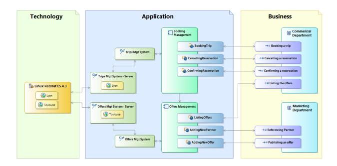
We look to replace the "Linux RedHat ES 4.3" component by the "Linux RedHat ES 6" component. The migration plan of improvements between the current architecture and the future one are represented by replacing at the Technology level the buggy server by the new one.
