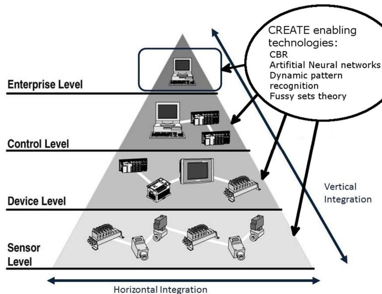
Figure 1. Automation pyramid and CREATE methodology.<sup>1</sup>
