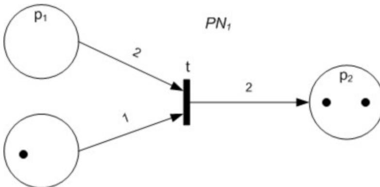
Figure 6. A Petri net from Figure 5 after a transition (marking 1)<sup>4</sup>
