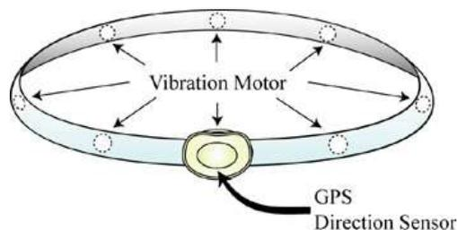
Fig. 6. Device for tactile feedback
