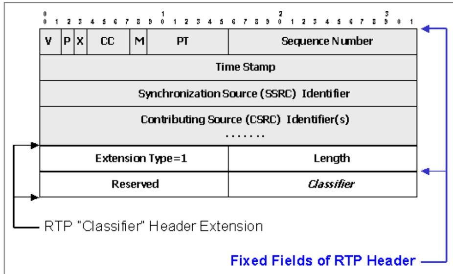
**Figure 3: RTP Header**
