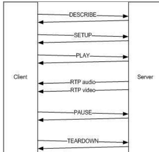
**Figure 4:** RTSP communication between server and client
