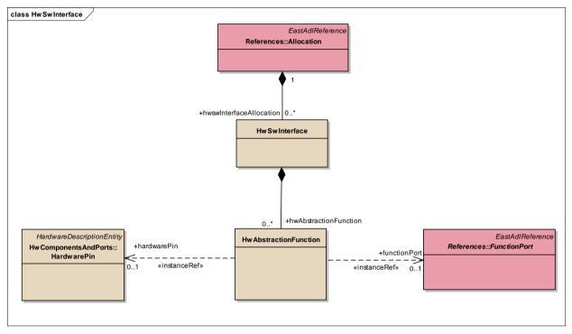
Figure 6: <u>**HwSwInterface**</u> - (*Class diagram*)
