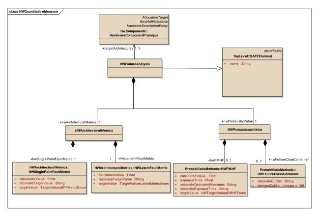
Figure 6: <u>HWQuantitativeMeasure</u> - (Class diagram)
