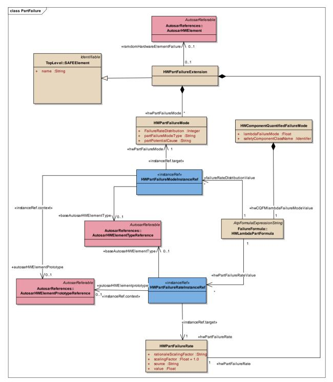
Figure 4: <u>PartFailure</u> - (Class diagram)
