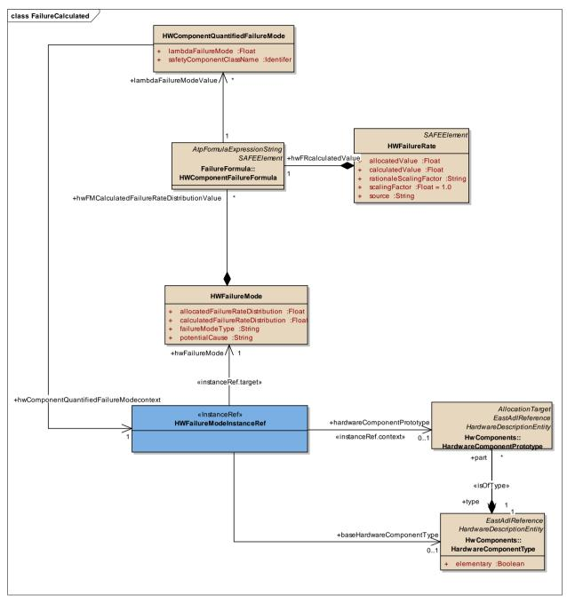
Figure 5: <u>FailureCalculated</u> - (Class diagram)
