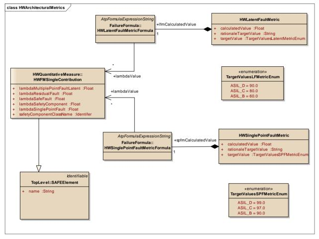
Figure 8: <u>HWArchitecturalMetrics</u> - (Class diagram)
