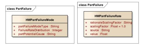
Figure 19: Hardware Part Failure information for IP-XACT
