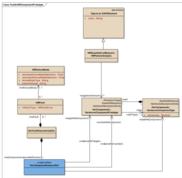
Figure 3: <u>FaultInHWComponentPrototype</u> - (Class diagram)
