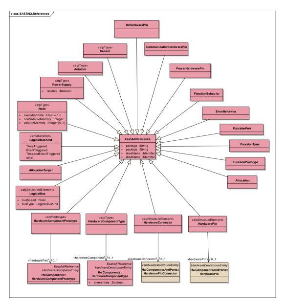
Figure 12: References of package Hardware to EAST-ADL
