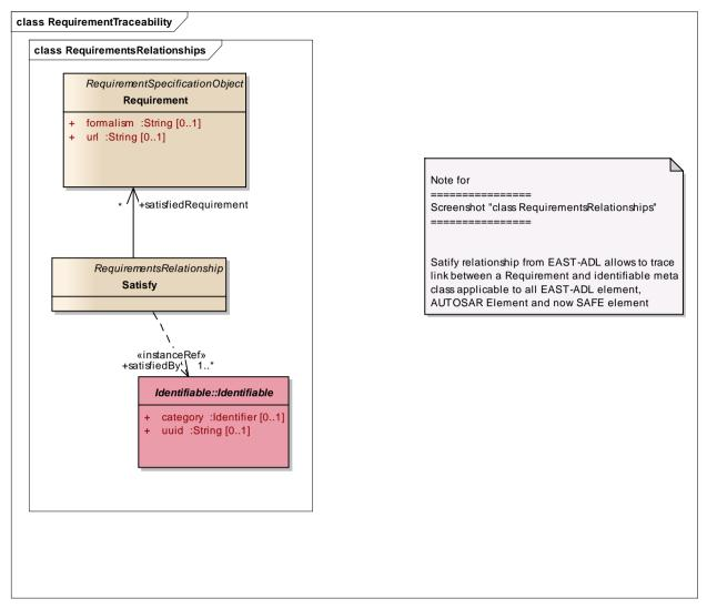
Figure 11: <u>RequirementTraceability</u> - (Class diagram)
