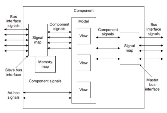
Figure 15: Structure of a component IP-XACT
