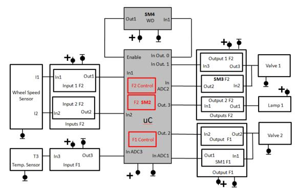
Figure 14: Technical Safety Concept for ISO26262-Part5 Figure E.1
