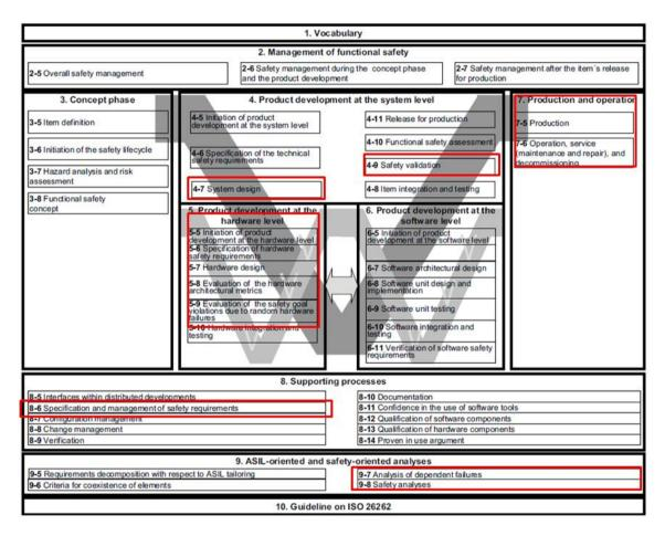
Figure 1: Overview on ISO 26262 (Relevant parts highlighted)
