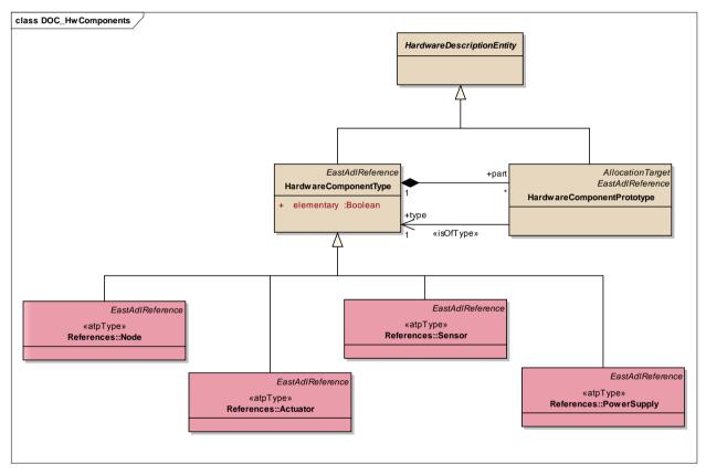
Figure 4: <u>DOC\_HwComponents</u> - (Class diagram)
