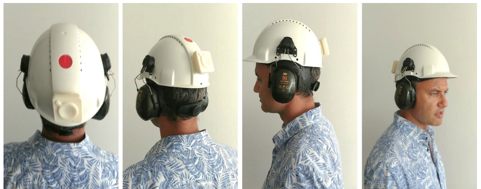
Safe Rescue - Personal tracking device conceptual prototype 2
