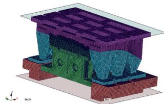
Simulation of the solidification of a break disc pattern (MAGMA)
